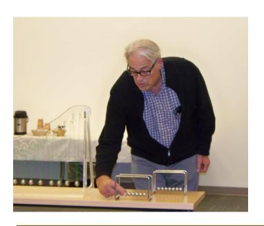
Rob Lieb has recently expanded the Newton's Cradle tabletop demonstration to include more pieces for students to use. The original cradle is still in use, but requires frequent "tuning" to get the ball positioned just right.. Another apparatus has been added to the demo (on left side of photo) that shows the harmonics when the balls are on different length strings.
